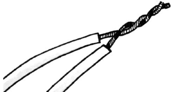
Step two: Hold the wires side by side and twist the exposed ends around each other.
